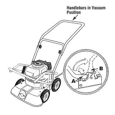
Figure 11: Handlebar position for vacuuming.
